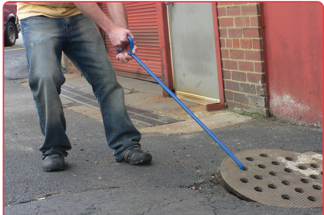
MANHOLE HOOKS ALSO ENGAGE VENT HOLES.
