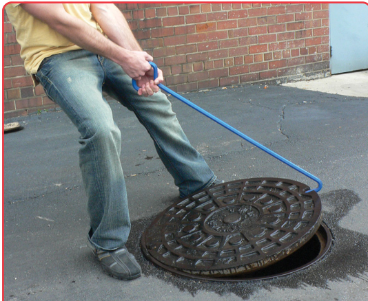
MANHOLE HOOKS ENGAGE PICK HOLES.
