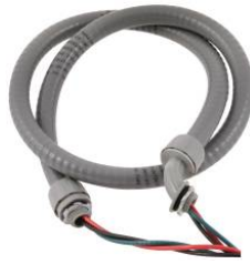
AIR CONDITIONER OR UNIT EQUIPMENT WIRING WHIP, 1/2 IN X 6 FT 3-#10 THHN
