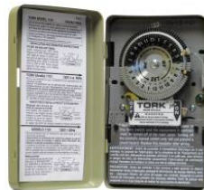
INDOOR TIMER SWITCH 24 HOUR SINGLE POLE METAL 2 HORSE POWER 40 AMP 120 VOLT
